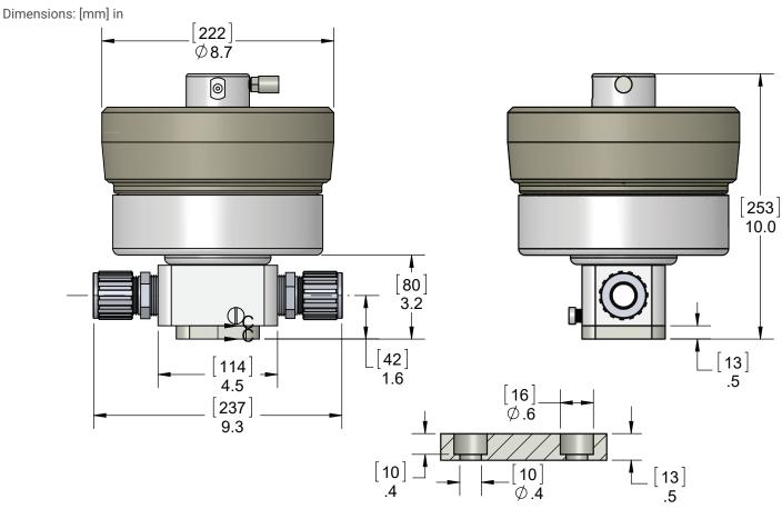
MAIN DIMENSIONS ARE INCHES, [BRACKETED] DIMENSIONS ARE mm.
