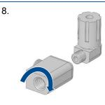
Attach 1/8" NPT elbow fitting to appropriate T fitting (T fitting must match pump air supply port, 3/8" NPT for 140 LPM series pumps, 1/4"NPT for 30 and 60 LPM series pumps)
