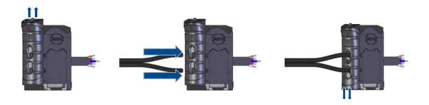
• Open the top and slide the front face of the D10 amplifier up. Press the fiber optic ends into the holes on the front face of the amplifier. Slide the face down to lock cables in place.
