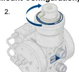
Attach dampener to pump via top check plug port, tighten to:
