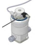
Lower ferrule and gripper to the probe. Hand-tighten the female gripper nut.
