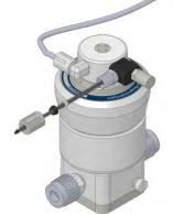
Insert the fiber optic cable into the leak detection probe - verifying that it makes contact with the bottom of the probe.
