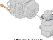
Affix air supply to T fitting attached to pump.
