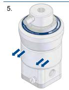
Place dampener onto mating base knobs. Slide dampener forward.
