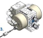
Insert the fiber optic cable until it contacts the bottom of the probe.
