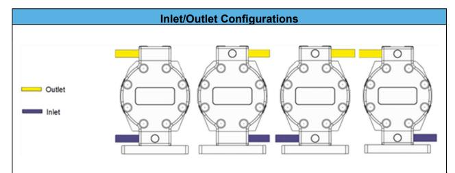
Some configurations require re-orientation of crossover manifolds. See Disassembly and Assembly Instructions.
