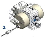
Insert the fiber optic cable until it contacts the bottom of the probe.
