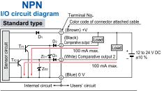
Symbols · · · D<sub>1</sub> to D<sub>3</sub> : Reverse supply polarity protection diode
