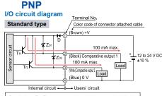
$$\label{eq:Symbols} \begin{split} \text{Symbols} \cdots D: \text{Reverse supply polarity protection diode} \\ Z_{D1}, Z_{D2}: \text{Surge absorption zener diode} \\ T_{C1}, T_{C2}: \text{PNP output transistor} \end{split}$$
