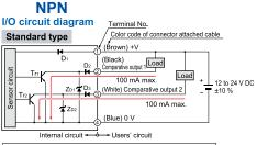
Symbols · · · D<sub>1</sub> to D<sub>3</sub> : Reverse supply polarity protection diode
