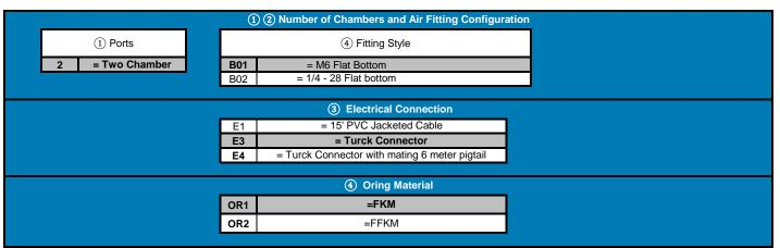
The following configuration has 2 Chambers, M6 flat bottom liquidn connections and turck connecters and FKM Orings;
