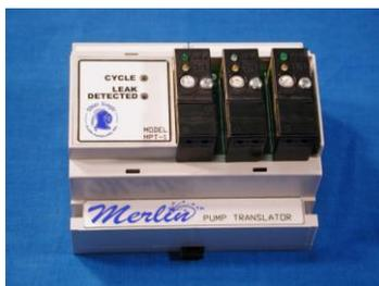
Merlin™ pump translator. Converts input from stroke detection to output of different fractional rate to allow for drop in replacement of other monitored pumps of different displacements.
