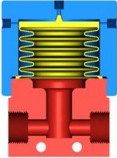
During stroke of the pump liquid pressure overrides air pressure and fills bellows with liquid.
