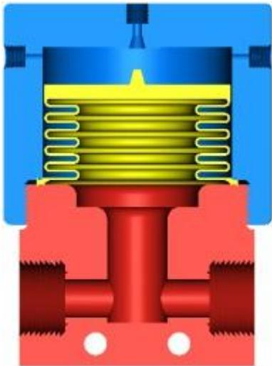
During shift of the pump air pressure overrides liquid pressure and moves liquid from bellows to outlet line to reduce line pressure delta.
