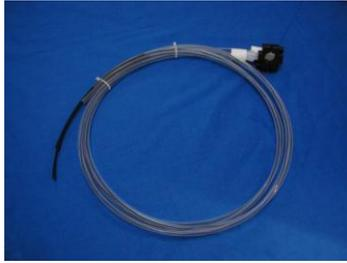
Bubble In – Bubble Out™ Fiber optic leak detection. Monitors inlet line for bubbles and outlet line for bubbles. If both have bubbles (as in priming or if chemistry is boiling) the monitor does not react. If there are no bubbles in the inlet line, but bubbles are present in the outlet line, a leak is assumed and alarm is sent.
