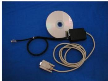
Hardware and software for programming Merlin™ pump translator from laptop or PC.
