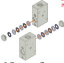
8. Remove muffler cap from left side using the muffler cap tool. Remove muffler media and note the order of the pieces. Repeat this step for muffler cap and muffler media on the right side.
