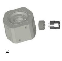
Use the appropriate PVC tool to remove the muffler from the pump body.
