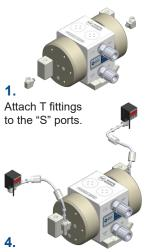
Loosen female gripper nuts on elbow assemblies and T fittings. Insert tubing and hand-tighten gripper nuts.
