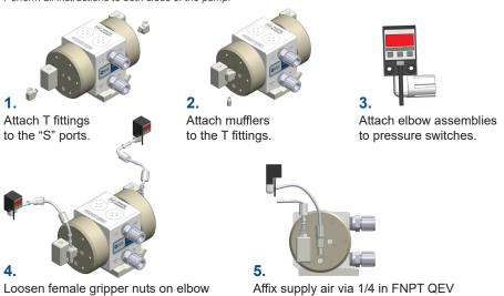
Loosen female gripper nuts on elbow assemblies and T fittings. Insert tubing and hand-tighten gripper nuts. Affix supply air via 1/4 in FNPT QEV ports on both sides. Air supply must be 1/4 in minimum orifice to source.
