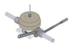
Torque liquid fittings to manufacturer spec. Use a backer wrench on fitting body.
