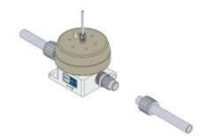
Loosely attach liquid connections.
