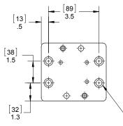
MOUNT WITH 4 3/8 [10mm] SOCKET HEAD CAP SCREWS—
