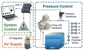
CPC-1 sends analog signals to an The regulator applies pressure to the pump. The pump pressurizes the fluid line. Sensors in the fluid line send analog signals to the CPC-1, which adjusts to repeat the process. The CPC-1 also communicates to external alarms, a PLC, or Windows-based computer, allowing it to integrate with various tools. https://wkfluidhandling.com/closed-loop
