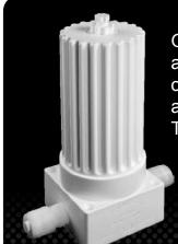
Gauntlet filter housings contain no metal parts and allow for changing filters without disconnecting inlet or outlet lines. They are ideal for high-temperature applications (up to 210°C). The patented Synchro-Thread® design utilizes face and diameter seals to provide reliable containment. The bellows and jack screw stabilize the filter in thermal cycling applications and allow for inverted installation.
