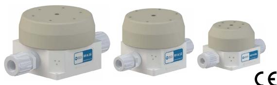
White Knight forward pressure regulators feature an air spring design that responds immediately and is highly accurate. They offer remote piloting capability to maintain system pressure for recirculation loops or systems with multiple tool drops or dispense points. They are available with 1/2 in. (RFA08), 3/4 in. (RFA12) and 1 in. (RFA16) connection sizes.
