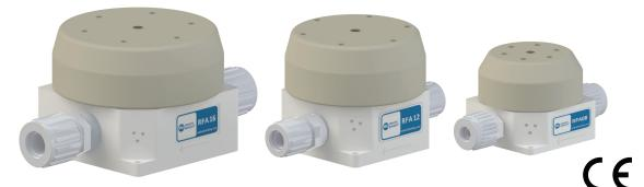
White Knight forward pressure regulators feature an air spring design that responds immediately and is highly accurate. They offer remote piloting capability to maintain system pressure for recirculation loops or systems with multiple tool drops or dispense points. They are available with 1/2 in. (RFA08), 3/4 in. (RFA12) and 1 in. (RFA16) connection sizes.
